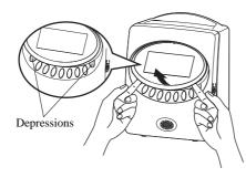
While pushing, turn the key to "O" position. At that moment, display will be as shown in the following figure. Then, you can go into the setting mode.
