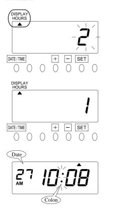
**1** Push the DATE/TIME button for 1 second and position the "A" under the "DISPLAY HOURS" mark.
