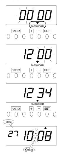
**Push the FUNCTION** button for 1 second, and position the " $\blacktriangle$ " over the "PASSWORD" mark.
