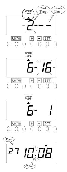
**1** Push the FUNCTION button for 1 second and position the " $\blacktriangle$ " under the "CARD TYPE" mark.
