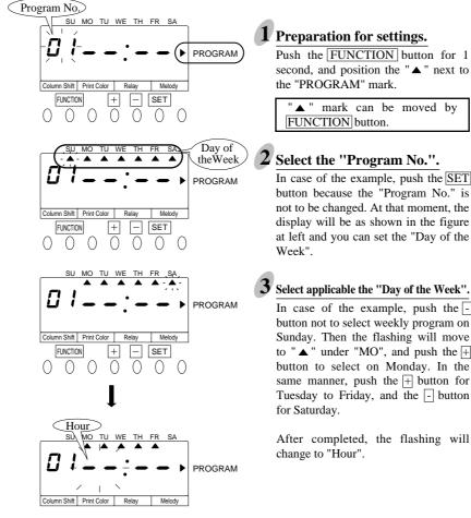
**Preparation for settings.** Push the FUNCTION button for 1 second, and position the "▲" next to
