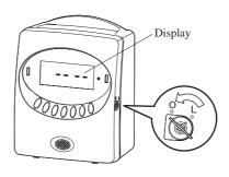
3 After the setting has been completed, push the <u>SETTING END</u> button to get out of the setting mode. Turn the key to "L" position. Make sure "date" and "time" are indicated on the display and colon is flashing. 4 Replace the cover. At that time, make sure to fit the tabs at the both side of the cover into the holes on the unit.
