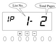
Push the \* and + button for 3 seconds. At that moment, "IP" is indicated on the left-side of display.
