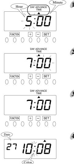
**1** Push the FUNCTION button for 1 second, and position the " $\blacktriangle$ " under the "DAY ADVANCE TIME" mark.
