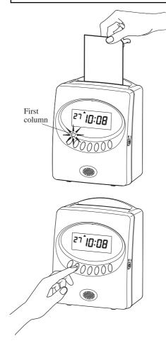
The clock can print time on the column under flashing lamp.
