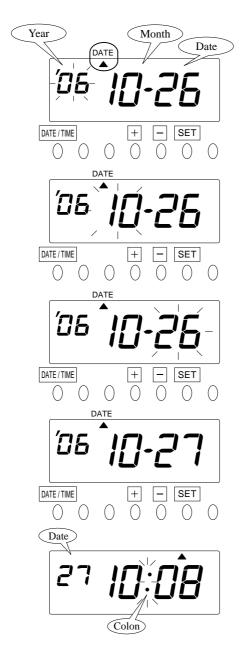
**1** Push the DATE/TIME button for 1 second and position the "A" under the "DATE" mark.
