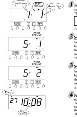
Push the FUNCTION button for 1 second and position the "▲" under the "PRINT FORMAT" mark.
