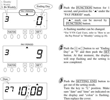
Push the FUNCTION button for 1 second, and position the " $\blacktriangle$ " under the
