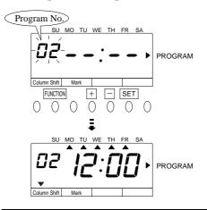
Push the + button and the "Program No." will start flashing. Push the + button once again to set the Program No. at "2".
